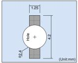
The recommended thickness of the screen mask for soldering is between 100 and 150 $\mu\text{m}.$  The hole size of the screen mask should be same as the recommended land pattern or smaller.
